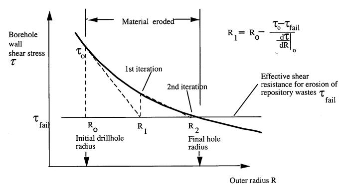
Figure 4. Iterate to find the final hole radius
