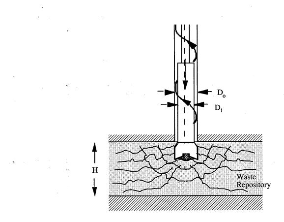
Figure 7 Fractured Waste Matrix after Penetration
